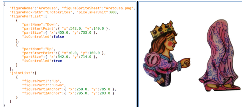
Fig. 6. Digital puppet representation. On the left, the json file describing how the puppet is composed of different parts, where these parts can be found in the corresponding sprite sheet and where the joint anchors are placed. On the right, the corresponding sprite sheet is depicted.
